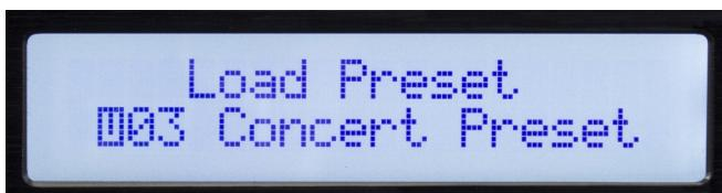
Rotate the Parameter knob to select the desired preset number then press to load.
