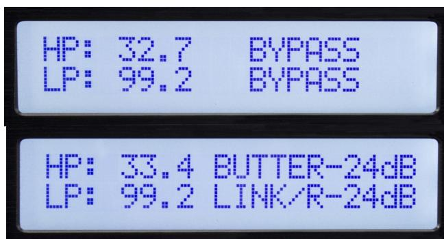
Although the button is labeled X-OVER and that is how these functions are often used, each input and output have very flexible high-pass and low-pass filters that can be configured for many applications.
