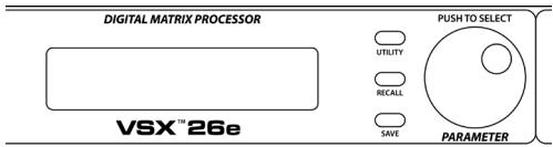
Pressing the utility button opens the screens for system wide settings. Each press of the utility button advances to the next screen in the sequence. You can press the "Exit" button at any time to return to the main screen.
