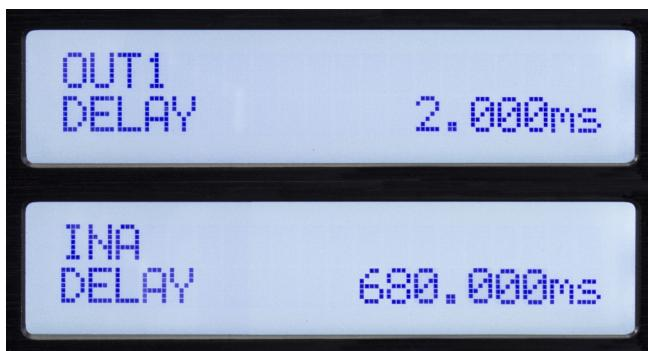
Up to 680 milli-Seconds of delay can be added to any input or output. The delay resolution is 1 sample or 10.4 micro-Seconds.
