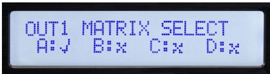
The Matrix screen is only available when editing an output. This is where the inputs that drive each output are connected. The above screen shows input "A" as the signal source for output 1. If multiple inputs are selected, their signals are summed.
