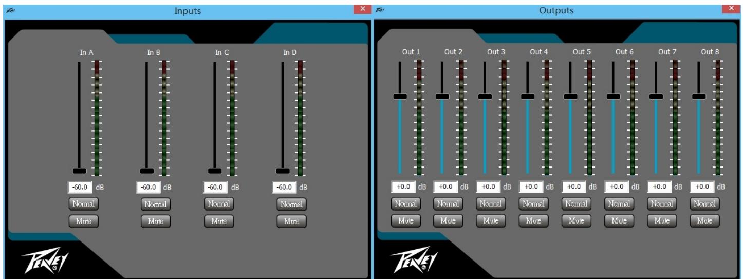
The gain screen above gives a good overview of the system. In addition to showing input and output gains, mute and polarity status, Input and output equalization curves can be displayed.
