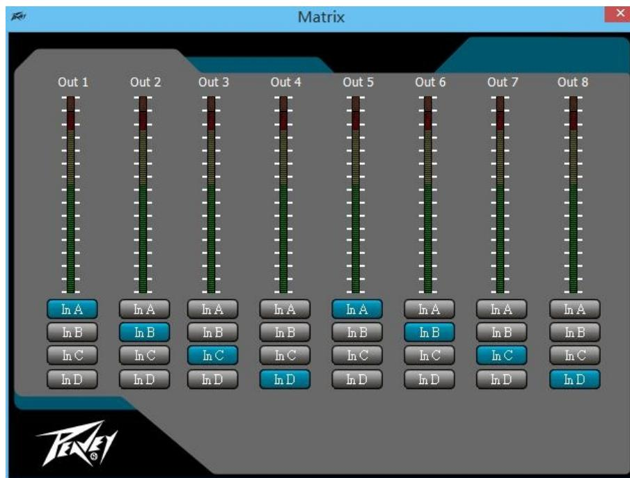
The input sources for each output are routed on the Matrix screen. Click the input button below the output to select. If more than one source is selected those inputs will sum. A graphical representation of the routing is given at the top. Inputs and outputs can also be labeled in this screen.
