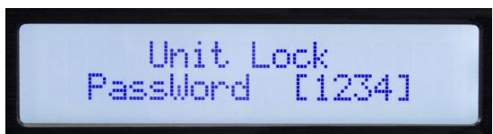
Once on this screen, the parameter knob is used to set the password. Press to advance and rotate to change each digit. A "Y" or "N" will appear allowing to engage the lock "Y" or turn it off "N".
