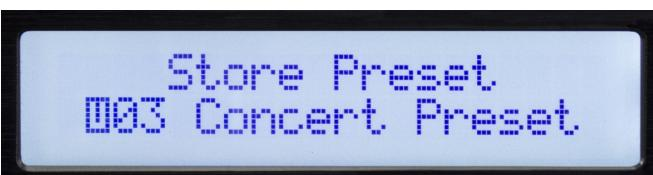
Select the desired user storage location using the parameter knob then Press. Enter a name for the preset and then press the parameter knob again when the "Y" appears to complete the save.
