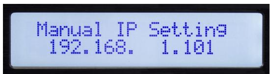
Set the Ethernet, IP address here for connection to the Editor program using the Ethernet port. Make sure to note the new address if you edit address!
