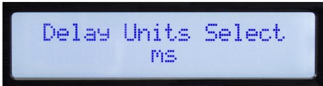
The units used to set delays can be selected on this screen. The options are milli-Seconds (mS), meters (m) or feet (ft)
