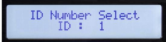
The ID number of the unit can be set in this screen. The ID is used with the Editor program to identify this unit when multiple units are connected. Each unit must have a unique identifier. It is most important when units are connected together using the RS 485 serial interface. See the section on serial communication for more details.
