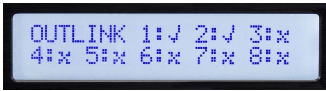
Many times, in particular for stereo signals, you may want to make the same adjust to two or more channels at the same time. Using the link function, inputs can be linked to other inputs and outputs can be linked to other outputs. The check marks on the above screen indicate linkage. When channels are linked, the edit buttons for those channels will blink simultaneously when editing.
