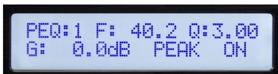
The input channels have 8 bands of equalization available and the outputs have 9. The EQ band is indicated in the upper left corner of the display. (Band 1 is shown above) The parameter selected for adjustment will blink on the screen. Press the parameter knob to select a parameter for editing. Rotate the knob to adjust.
