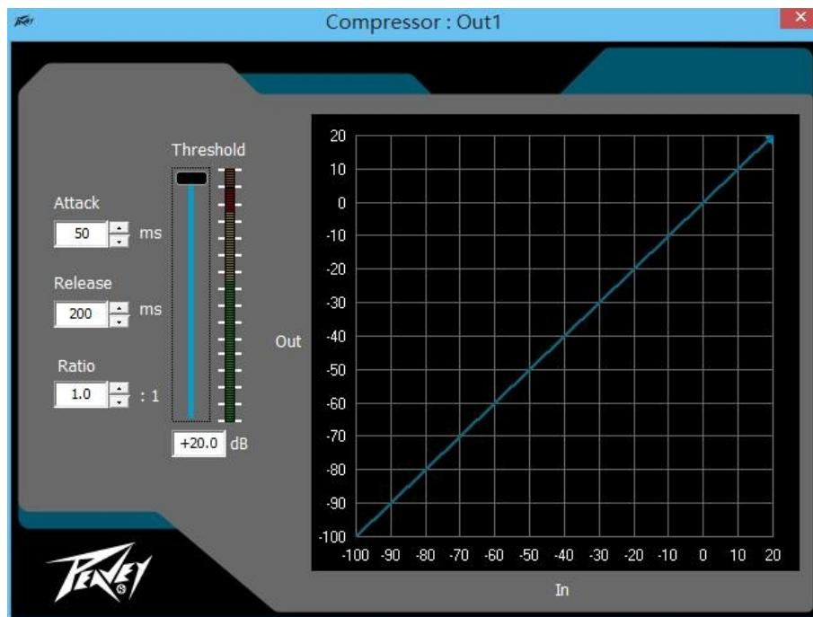
The Compressor screen displays the settings of all 8 output compressors along with signal level, and limit status. The transfer function of a selected output is also displayed.
