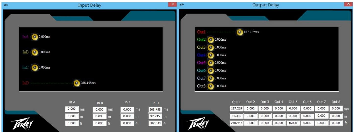
All of the input and output delays are shown in the above screen. Delays can be adjusted using the sliders at the bottom, by sliding the speakers at the top or by direct typed entry. To directly enter the delay time, double click the delay time and type a new value. If you hold down the left mouse button on a slider, you can fine adjust the delay by using the up and down arrow buttons on the keyboard.
