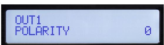
0= Normal polarity. 180= Reverse polarity.
