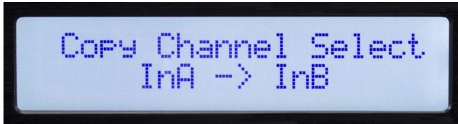
Settings can easily be copied from one input channel to another input or from one output to another. Rotate the parameter encoder to select the parameter.
