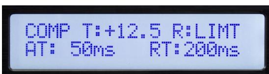
The compressor screen is only available when editing an output. The compressor parameters are: T= Threshold, R= Ratio, AT= Attack Time and RT= Release Time. The threshold is roughly equal to the limiting level in dBu. The limit LED corresponding to the output channel will light when the threshold is exceeded. The status is also displayed in the computer editor.
